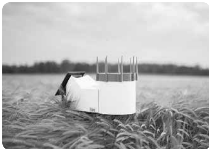
Regenmesser der Fasterrain Station.
